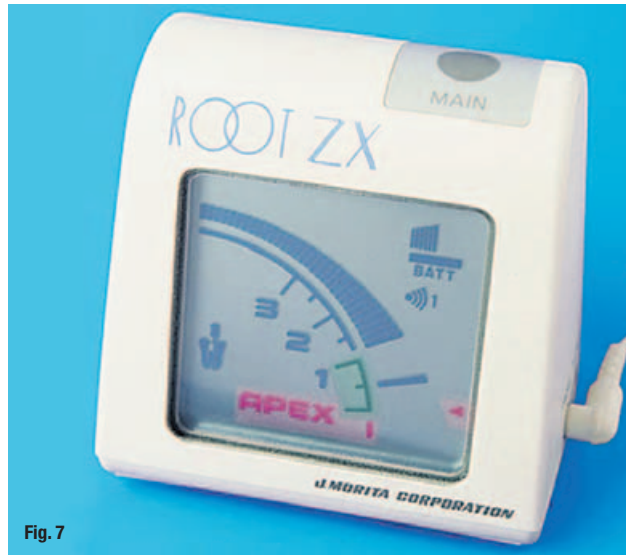
Fig. 7_ The Root ZX is a fully automatic, self-calibrating root canal foramen locator.
